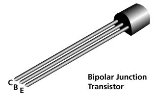
A typical Bipolar Junction Transistor (BJT) has three terminals attached to a plastic body. The body has a flat side. The terminals can be recognized by their position on the body. With the terminals pointing towards you and the flat side pointing away from you, the right terminal is the emitter (labeled E in the diagram), the middle terminal is always the base (labeled B in the diagram), and the left terminal is the collector (labeled C in the diagram).
